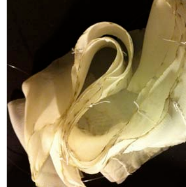
03. Synthetic textile, double layers lasercut simultaneously (welded together), sewn
