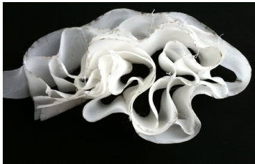
02. Chiffon, laser cut, sewn Chiffon not structural enough, sewn seams affect surface behaviour but do not create volume in assembly.
