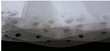
06. Translucent 0.8mm Polypropylene, laser cut and perforated, tied assembly
