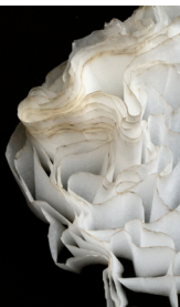
04. Tissue paper, laser cut, glued No distortion in Z-direction. Distortion of grid in X & Y direction results in structure no longer fully retractable due to differing member lengths. Flexibility of material means structure lies flat - assembly is not inherently volumetric.
