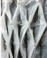
03. Synthetic textile, double layers lasercut simultaneously (welded together), sewn
