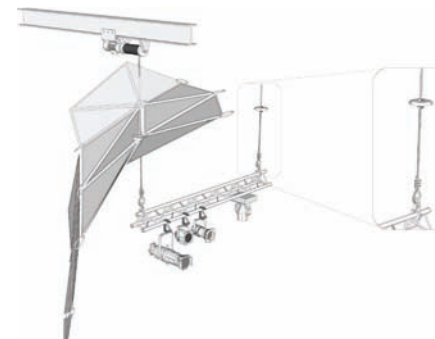
Detail of Carpet Tile Structure and Lighting System
